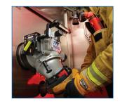
Connecting the LDH is easier. The swivel allows the elbow to twist with the charging LDH from the fire hydrant.
