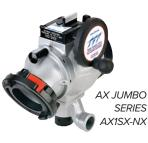
TFT's Jumbo Ball Intake valve has a huge 5.25" (133mm) diameter waterway giving low friction loss to maximize flow. Friction loss is 3 psi at 2000 gpm (0.2 bar @ 7600 l/min). Designed for use with 3.5", 4", 4.5", 5" or 6" (89, 100, 115, 125 or 150mm) hose. A parallel shaft handle is also available for a top mount control for minimal interference.
