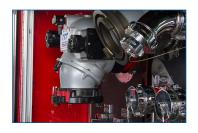
Industry standard of a 5.25" (133mm) waterway. The unobstructed waterway on a BIV with a 5" (125mm) coupling has only 11 psi loss at 2000 gpm (0.7 bar @ 7600 I/ min) and there's only 3 psi of loss at 2000 gpm (0.2 bar @ 7600 I/min) for the Jumbo Valve series with a 6" (150mm) coupling.
